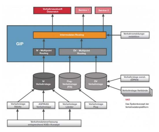
Figure 2: System structure of traffic information in Austria (Source: <u>http://www.gip.gv.at/vao-technische-details.html</u>)
